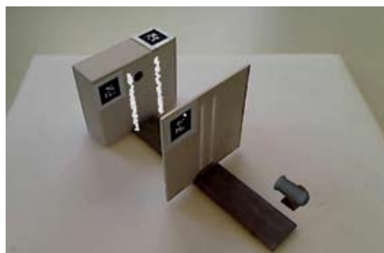
Figure 6. The double slit setup consisting of a floor board (dark), the slit board in the foreground, a box as a projection plane, and a virtual cannon
