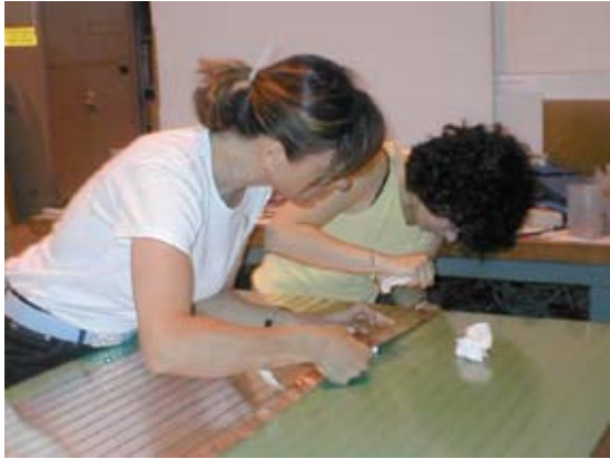
Figure 3. Making a readout plane: Glueing copper strips on a vetronite sheet.
