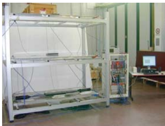
Figure 7. A muon telescope on its support frame in the Gran Sasso laboratory.
