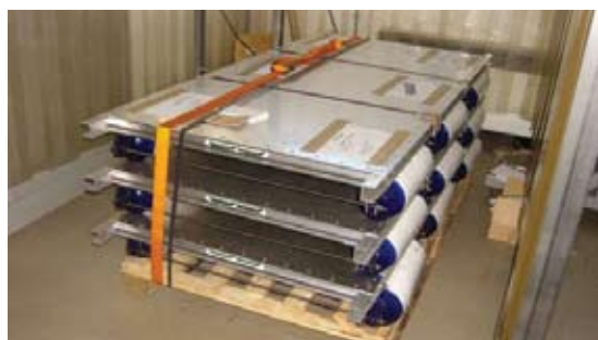
Figure 6. The 3 MRPCs of a muon telescope, inside their aluminium boxes, packaged with boat fenders for safe transport.
