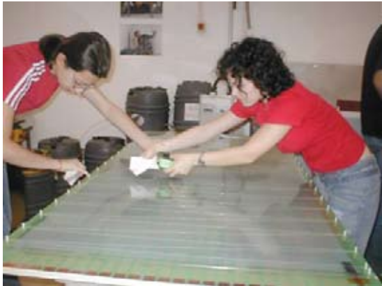
Figure 4. Stretching the fishing line spacer in a zig-zag pattern between glass plates.
