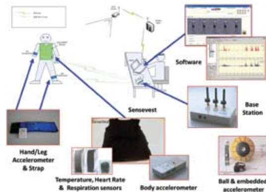
Figure 2. General architecture of the KLiC system and its sensors.
