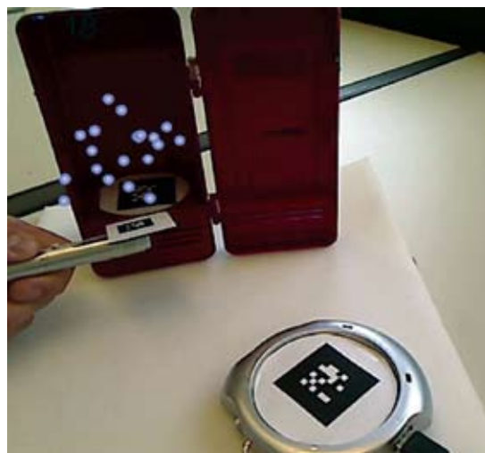
Figure 9. The Boltzmann exhibit: Heating plate in the front refrigerator in the back. The user holds the thermometer into an area of low energy and recognizes a slower movement of the molecules.
