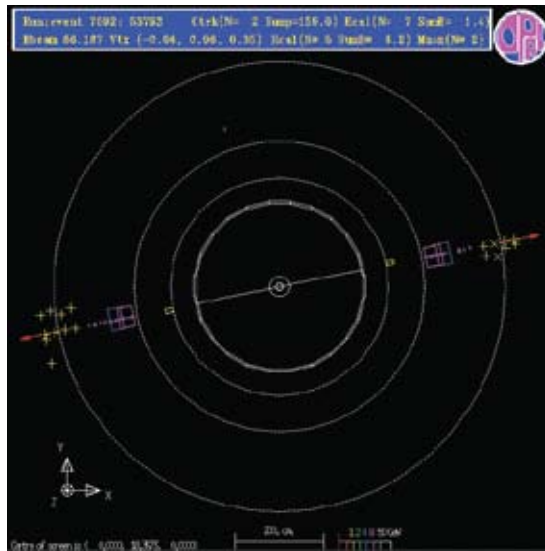
Figure 1. Example of e^+e^- \rightarrow \mu^+\mu^- event from the OPAL experiment at LEP.
