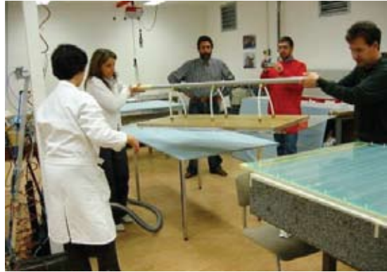
Figure 5. Lifting a glass plate with a vacuum system to position it on top of the previous one.
