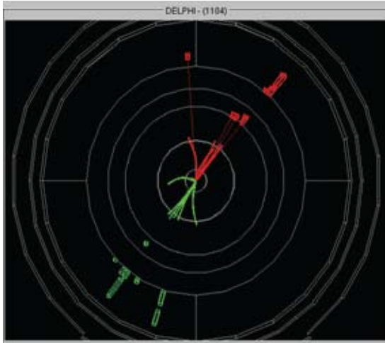
Figure 1. Display of a Z-decay event from the DELPHI detector in LEP of the sort that students analyze. This event is a candidate for a Z0 decaying into jets of hadrons.
